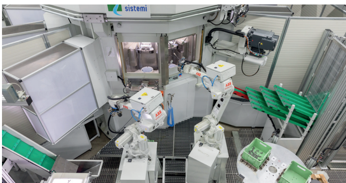
Fully automated STAUFF fittings production
